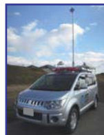
←New portable satellite model Not only downsized but also the added an automatic satellite signal lock-on/tracking function.
