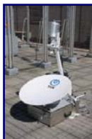
←New portable satellite model Not only downsized but also the added an automatic satellite signal lock-on/tracking function.
