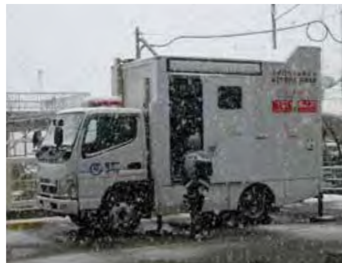
Portable satellite device connecting emergency use public phones at an evacuation center during a snowstorm (Iwaizumi Town, Iwate Prefecture)
